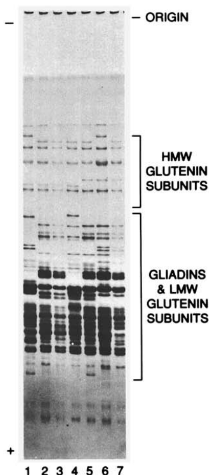
Fig. 2. Conventional sodium dodecyl sulfate gradient polyacrylamide gel electrophoretic separation of wheat storage proteins. The Canada Western Red Spring wheat cultivars analyzed include: Marquis (1), Neepawa (2), Conway (3), Columbus (4), Lancer (5), Laura (6), and Roblin (7). Storage proteins were divided into the two groups: high molecular weight (HMW) glutenin subunits; and low molecular weight (LMW) glutenin subunits and \omega -, \alpha -, \beta -, and \gamma -gliadins.
