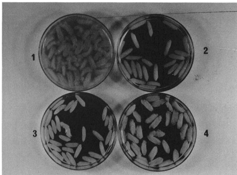
Fig. 1. Canning stability of rice modified by different cross-linking reagents. 1, parboiled (control); 2, epichlorohydrin; 3, sodium trimetaphosphate; and 4, phosphorus oxychloride.
