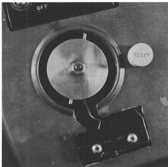
Fig. 5. Arrangement of cams and microswitch on sampler module. The top cam controls the automatic valve and is positioned relative to the bottom cam underneath (not shown) so that the change in buffers occurs at their point of mixing with the substrate (see Fig. 3) while the wash water aspirated between samples is combined with the substrate solution.
