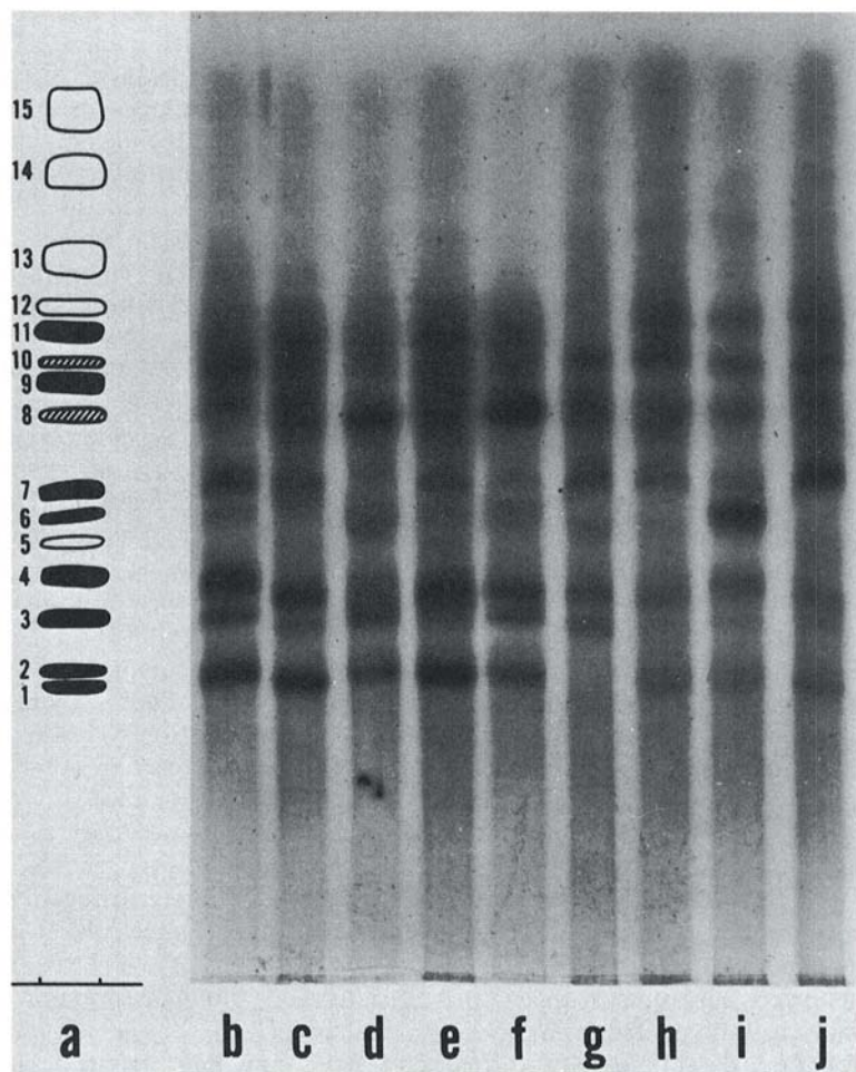
Fig. 7. SDS-polyacrylamide gel of glutenin from several varieties and classes: a) diagram and numbering system used in text for Ponca glutenin subunits, with prominent bands shaded; b) Ponca (hard red winter); c) Red Chief (hard red winter); d) Comanche (hard red winter); e) Selkirk (hard red spring); f) Red River 68 (hard red spring); g) Wells (durum); h) Omar (club); i) Brevor (soft white winter); and j) Seneca (soft red winter).
