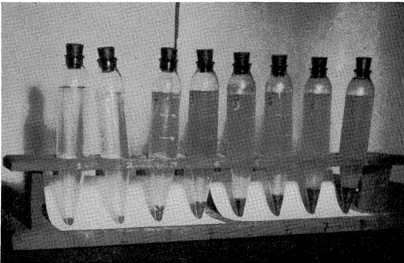
Fig. 4. Smut sediment formed 10 minutes after addition of Roccal. Tubes 1 and 2 represent no smut; 3 and 4, low; 5 and 6, medium; and 7 and 8, heavy smut.
