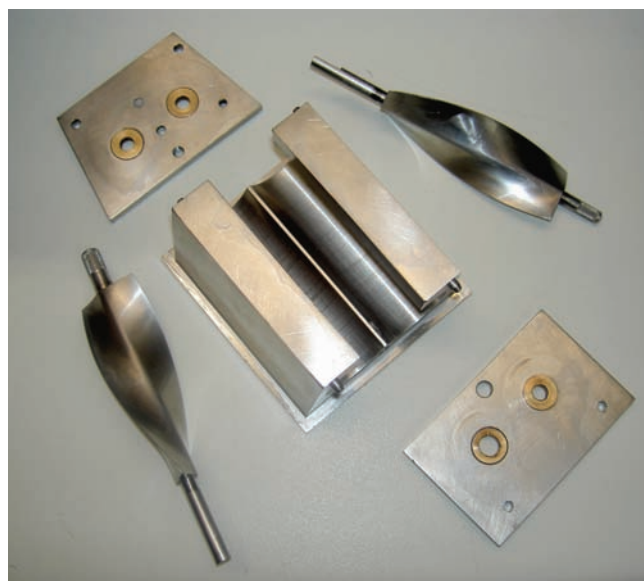
Fig. 3. The Mixolab dismantled.
