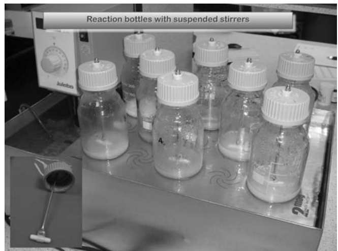
Fig. 3. Picture showing a 2mag Mixdrive 15 submersible magnetic stirrer in a custom made water bath. This allows stirring of 15 samples at controlled speed and 37°C.
