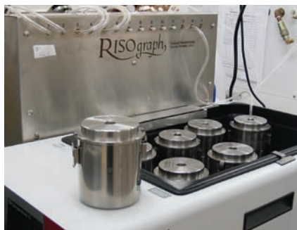
Fig. 3. Risograph equipment. This model will accommodate 12 sample containers plus the “M” measuring reference container, though only six containers are shown.
