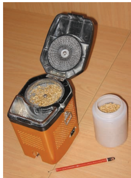
Fig. 1. The Kett Pearlest rice pearler, fitted with highly abrasive disk and rotor, suitable for wheat grain pearling.
