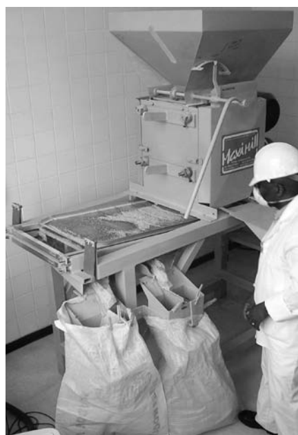
Fig. 3. Roller mill tested for sorghum milling at the University of Pretoria. The mill comprises two pairs of rolls and a sieving assembly.
