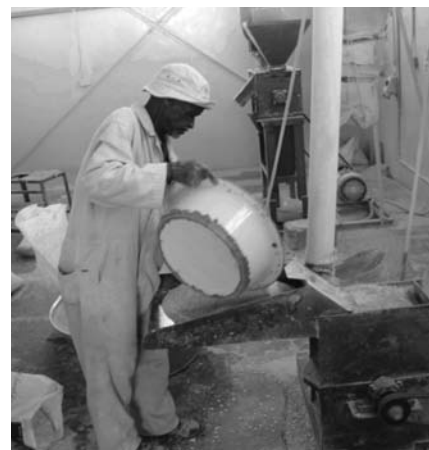
Fig. 2. Small sorghum mill in Botswana. Foreground, hammer mill; background, Prairie Research Laboratory type of dehuller.
