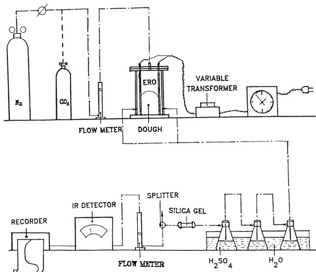
Fig. 2. Electric resistance oven system to detect rate of CO<sub>2</sub> loss.
