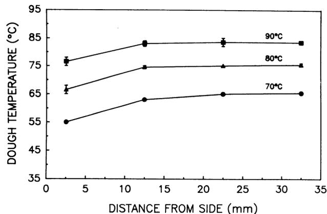
Fig. 10. Temperature gradients along the length and width of dough at a depth of 22.5 mm, when the temperature at the dough 10 mm above the bottom reached 70, 80, and 90°C.
