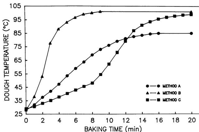
Fig. 4. Comparison of heating methods in temperature-time profile. Method A, 75 V (0–22 min); method B, 120 V (0–22 min); method C, 50 V (0–8 min), 90 V (9–10 min), 100 V (11–12 min), and 120 V (13–22 min).
