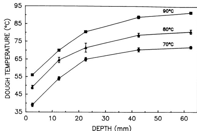
Fig. 9. Temperature gradients at different depths of dough, when the temperature at the bottom of the dough reached 70, 80, and 90°C.
