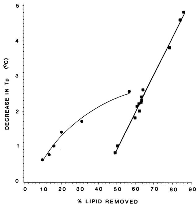
Fig. 3. The relationship between the decrease in  $T_p$  values and the percentages of nonstarch lipids removed from unmilled (●) and 1.3–9.1% milled (■) kernels. Data points are included for extraction times other than 25 min and 1 hr. Additional points on curve for unmilled kernels are for 15-min, 2-hr, 4-hr, and 8-hr lipid extraction times. Lowest point on curve for milled kernels is for 1.3% milled rice kernels that were solvent extracted for 15 min.
