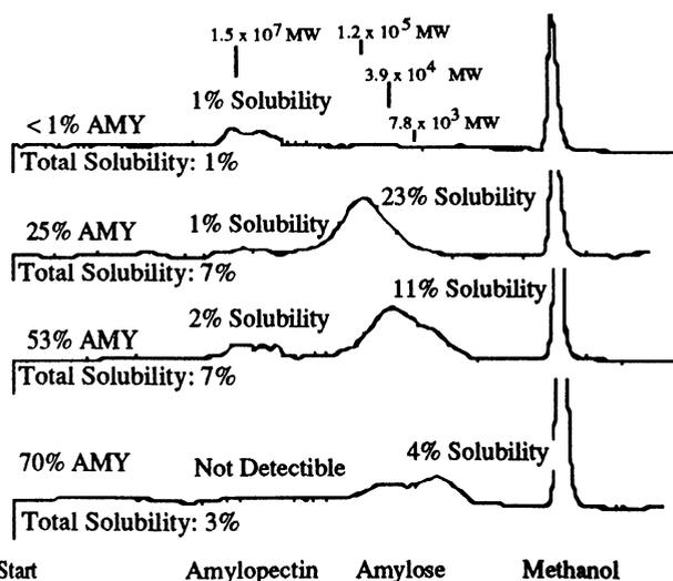
Fig. 1. High-performance size-exclusion chromatography solubility profiles of corn starch (1% solutions) extracted at 85°C by aqueous leaching for 1 hr. Data include total starch solubility, solubility of amylose (AMY) and amylopectin (AMP), and apparent molecular weights (MW).
