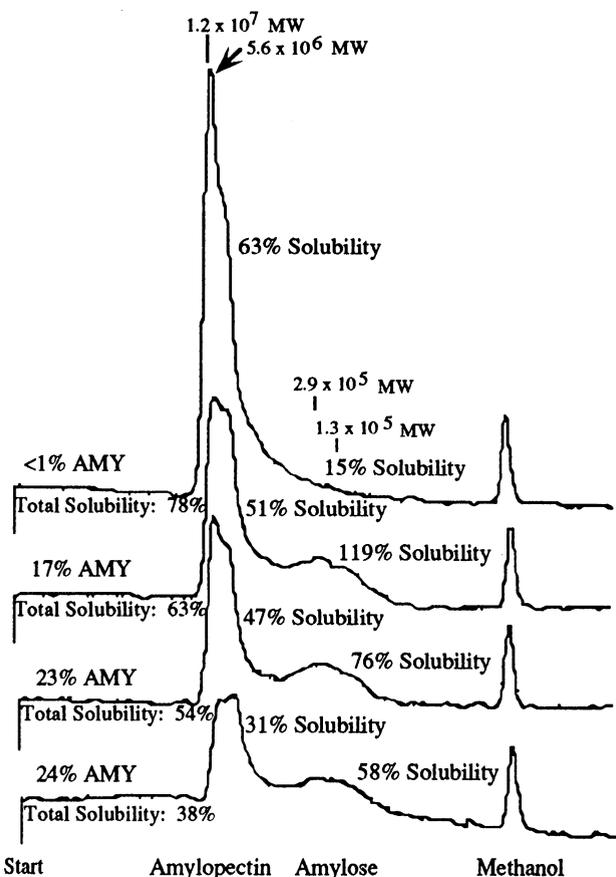
Fig. 6. High-performance size-exclusion chromatography solubility profiles of sorghum starch (1%) extracted at 85°C for 10 min and sonicated 20 sec. Data include total starch solubility, solubility of amylose (AMY) and amylopectin (AMP), and apparent molecular weights (MW). AMY solubility includes low-MW AMP. The amount of soluble low-MW AMP from waxy starch (<1% AMY) is presented.
