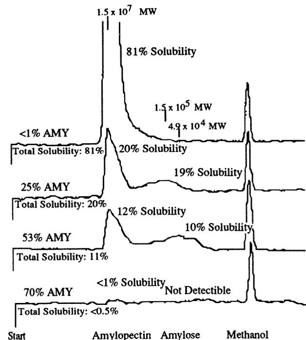
Fig. 4. High-performance size-exclusion chromatography solubility profiles of corn starch (1%) extracted at 85°C for 10 min and sonicated 20 sec. Data include total starch solubility, solubility of amylose (AMY) and amylopectin (AMP), and apparent molecular weights (MW).
