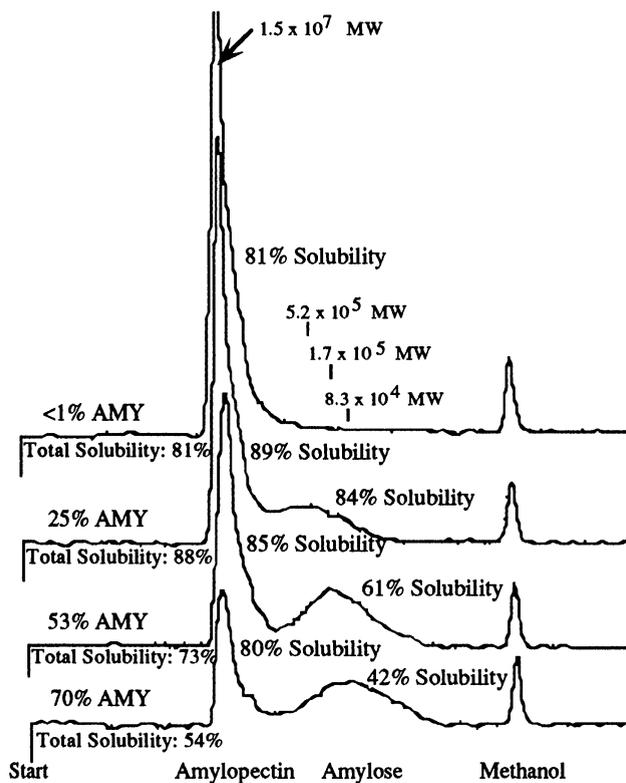
Fig. 5. High-performance size-exclusion chromatography solubility profiles of corn starch (1%) boiled for 10 min, autoclaved for 10 min, and sonicated 20 sec. Data include total starch solubility, solubility of amylose (AMY) and amylopectin (AMP), and apparent molecular weights (MW).
