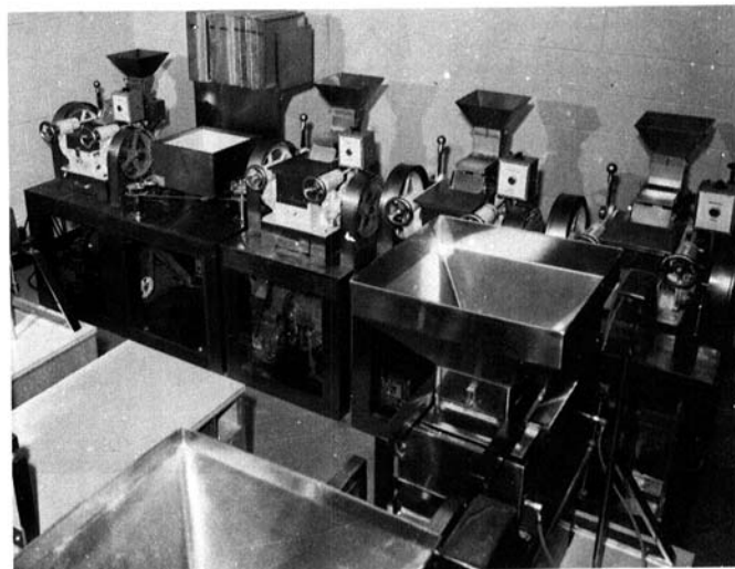
Fig. 1. The Grain Research Laboratory 6-in. (152-mm) laboratory research mill.
