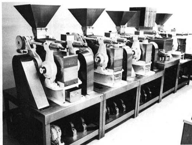
Fig. 2. The Grain Research Laboratory 10-in. (254-mm) laboratory research mill.
