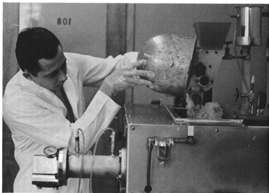
Fig. 1. Continuous press for extruding spaghetti on a semicommercial scale (25 lb. per hr.). Extrusion conditions can be controlled to produce spaghetti that is comparable to commercially processed products.
