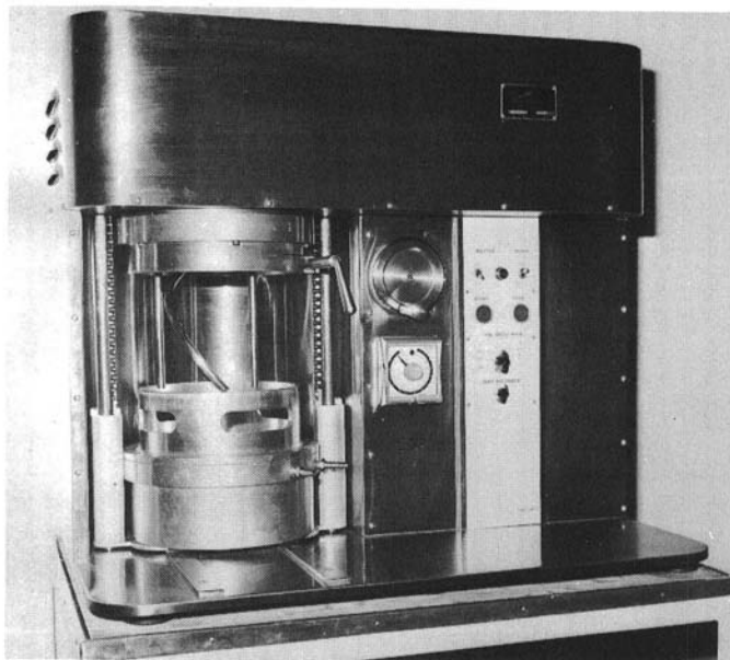
Fig. 1. The GRL-1000 laboratory dough mixer with mixing bowl in "down" position.
