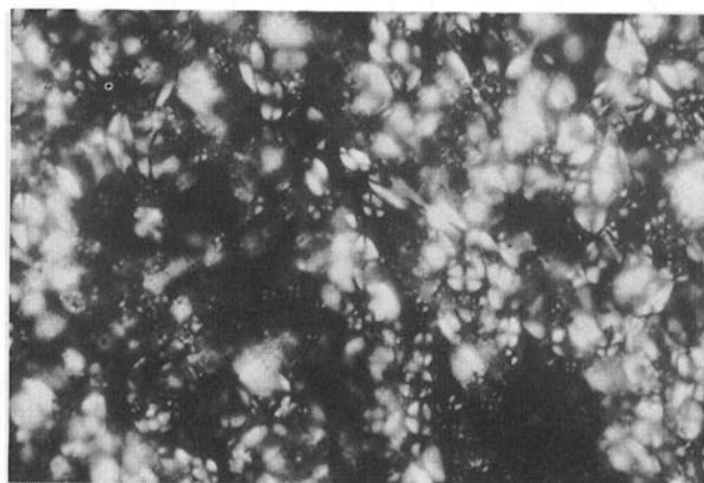
Fig. 3. Birefringent starch granules in straight doughs (polarized light, 250X).
